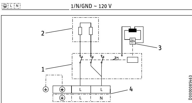
1 Power PCB with integral safety switch
