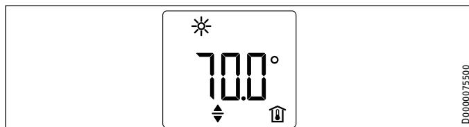
The standard display is continuously shown. If no user input is detected for longer than 20 seconds while in the menu, the device automatically switches to the standard display.
