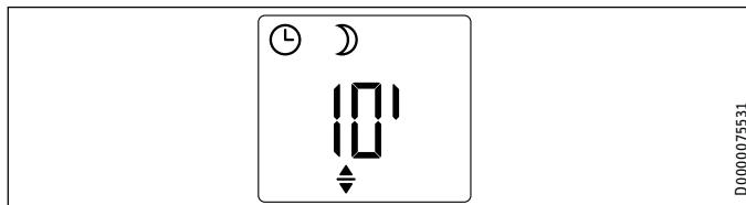
The standard display shows the selected time in minutes as well as the “Editable parameter” symbol. Using the “+” and “-” buttons, you can select any length of time from 10–120 minutes.
